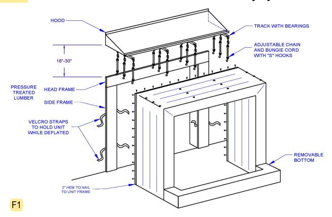
Figure 2: A four-sided MRI AIR shelter has a removable bottom that is connected to the side frames with velcor.
